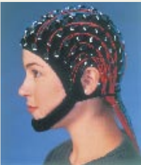
Illustration 2: A subject wearing an EEG cap fitted with 128 electrodes.
